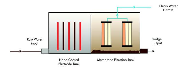
Utopia Eclear Unit Treat Water in two stages, first stage consists of Nano coated base electrochemical process and second stage consists of Advanced Membrane Unit. The first stage nano electrochemical process helps to remove organic and biological impurities with very low energy requirement.
